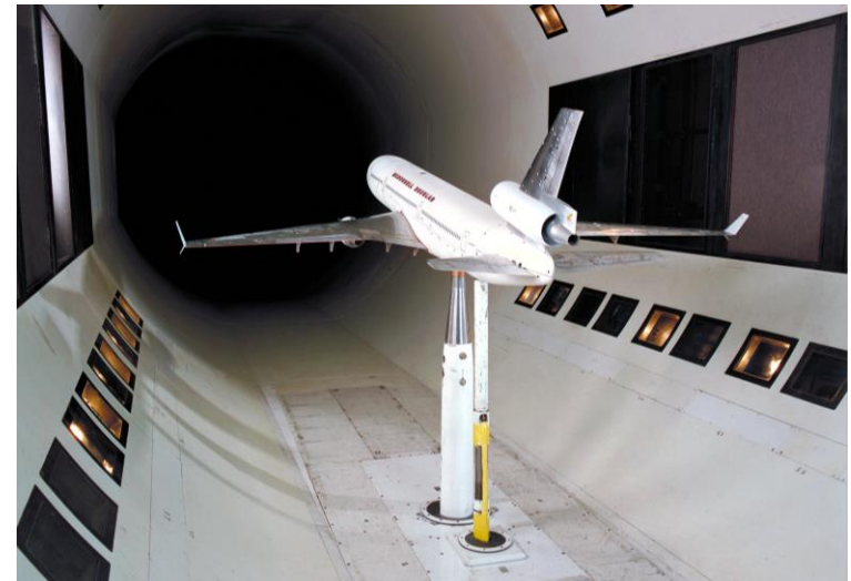
NASA wind tunnel with the scale model of an airplane
